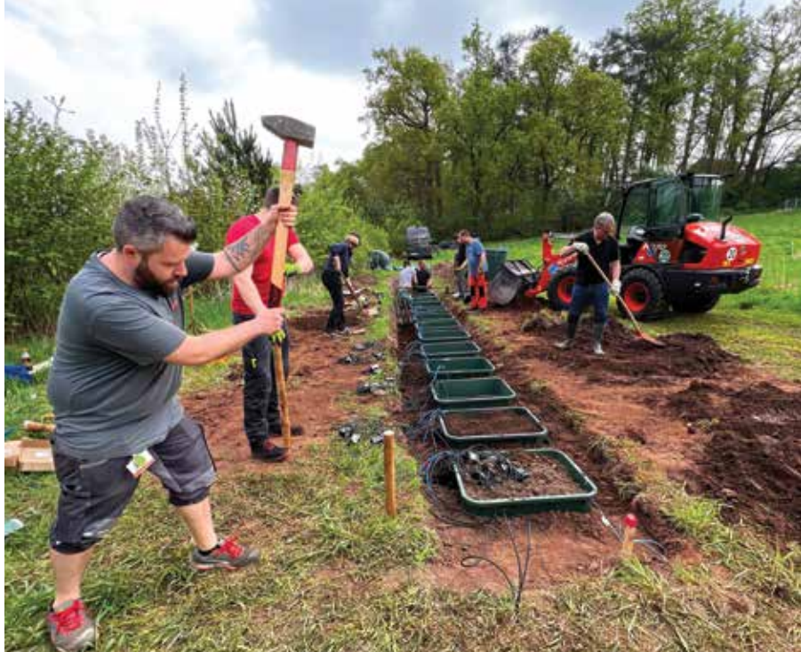
Researchers in Germany install devices for measuring the weathering process in a field trial of enhanced rock weathering. One sticking point with enhanced rock weathering is how best to measure and verify carbon capture.
